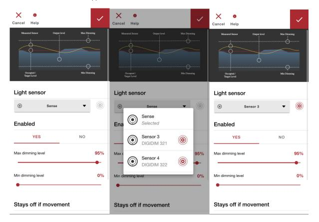
Note: Changing the light sensor will reset current DLH target level and starts automatic target calculation.
