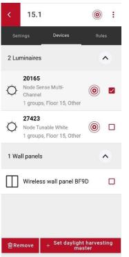
Daylight harvesting function is enabled by default on individual luminaires. To achieve an evenly dimmed ceiling, a group daylight harvesting master can be selected.
