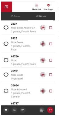
"Main screen" is the central view to navigate through the nearby devices and groups in the connected network. Here you can find a tab with a list of the discovered devices and another tab with a list of discovered groups. Filtering options are located at the bottom of the view.
