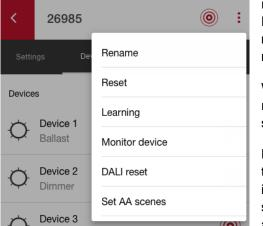
re-initialize DALI devices and DIGIDIM sensors attached to its DALI bus. This can be done through the three dots in the topright corner of the device details screen, by selecting "DALI reset" in the menu.
