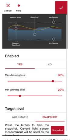
Purpose of the daylight harvesting (DLH) is to reduce the usage of artificial light when natural light is available. Light sensor measures the amount of light reflecting from the surface right below the sensor, so the luminaire can respond to the amount of natural light in the space by dimming the light, which helps to save energy and at the same time maintain the lighting level optimal for the user.
